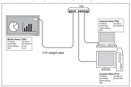
$<sup>\</sup>ensuremath{\mathscr{I}}$  When the monitor is connected to the computer directly without hub, the UTP cross cable should be used .
